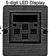
Operating-/Error display Normal - "LED on" Error - "LED blinks"
